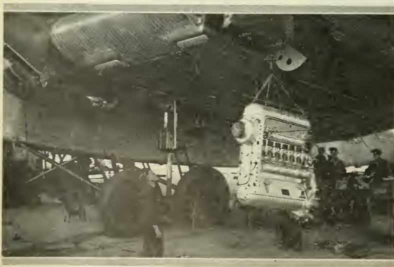
Installing one of the four Junkers Juno-4 engines in a G-38 transport plane
